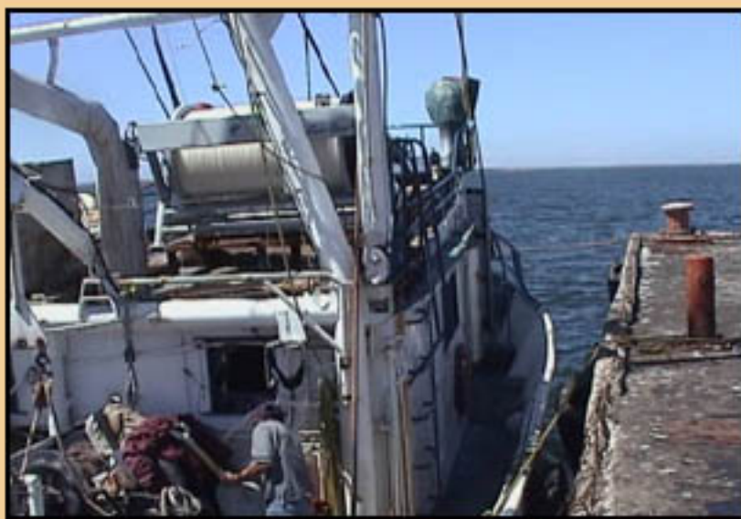
With the new Lingren/Pitnarm Super Spool any boat 50 feet or more in length, like the one pictured, can put a 50-mile, 2000 hook longline on their boat, when not so long ago it took a 100 foot boat to manage such an endeavor.
